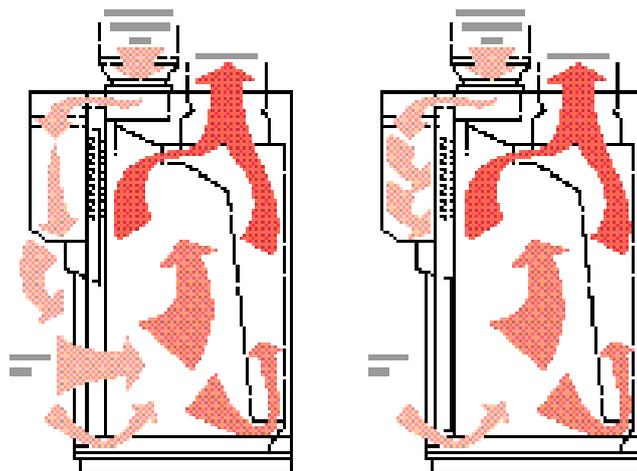
***Figure 3. Auxiliary cabinet with sash open & closed***
