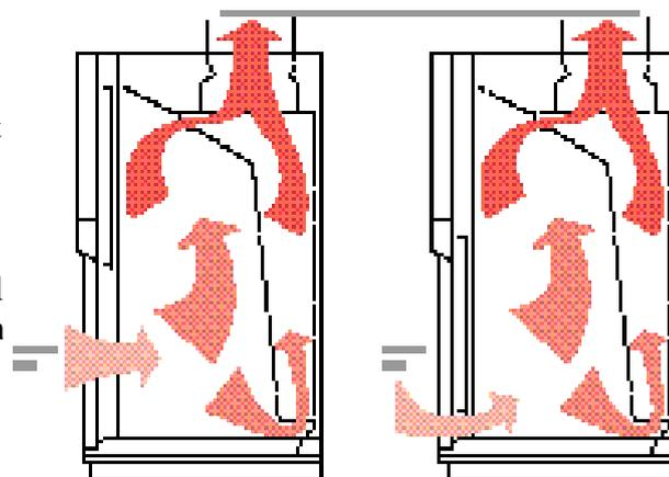
Figure 1. Conventional cabinet with sash open & closed
