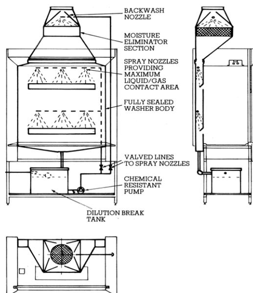
***Figure 5: Perchloric Fume cabinet extract system***
